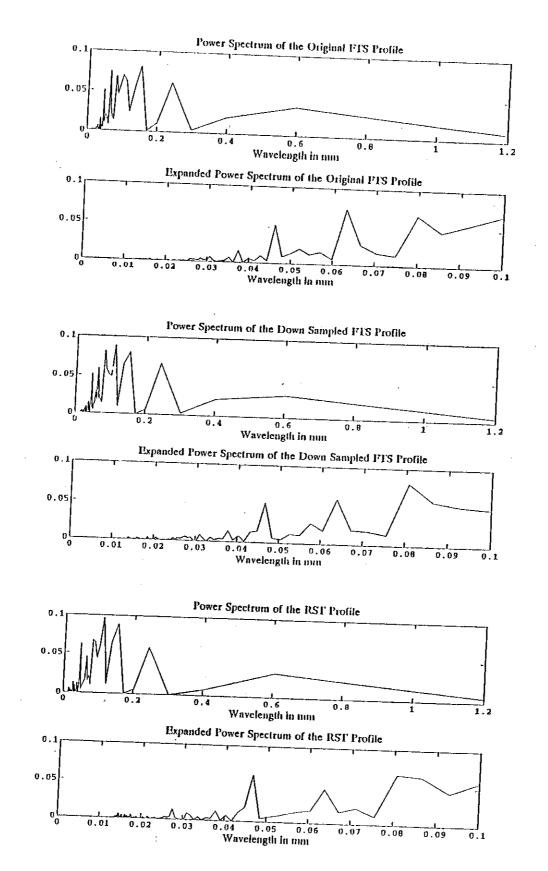
Figure 2. Power spectrum plots of profiles from PTB specimen
