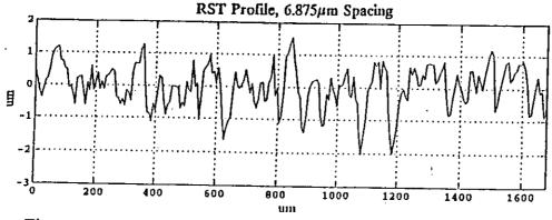
Figure 1. Unfiltered surface profiles from PTB roughness specimen
