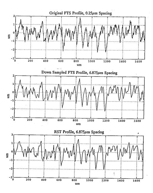
Figure 7 - Unfiltered surface profiles from PTB specimen.
