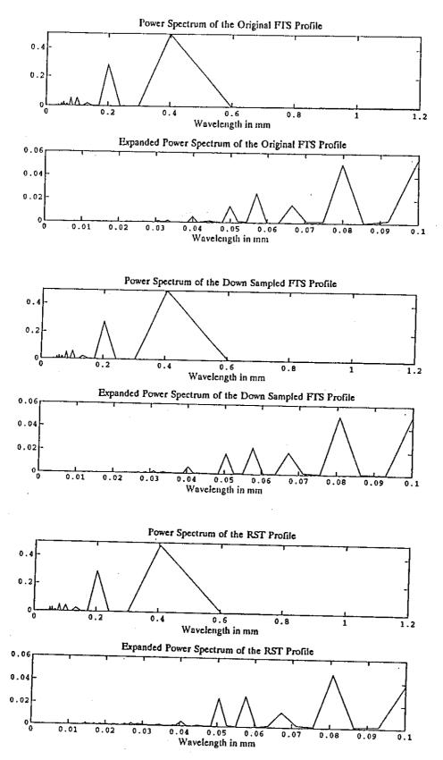
Figure 12 - Power spectrum plots of the milled surface profiles.
