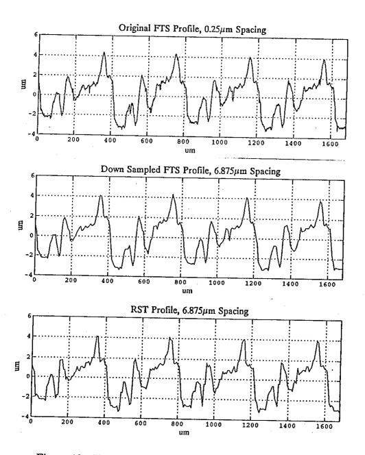
Figure 10 - Unfiltered surface profiles from the milled surface.
