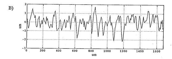
Figure 2 - Original (A) and down sampled (B) profiles at  $0.25\mu m$  and  $6.875\mu m$  ordinate spacings (PTB specimen).
