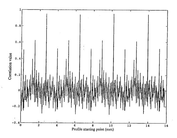
Figure 1 - The correlation values generated by the automated down sampling procedure (PTB specimen).
