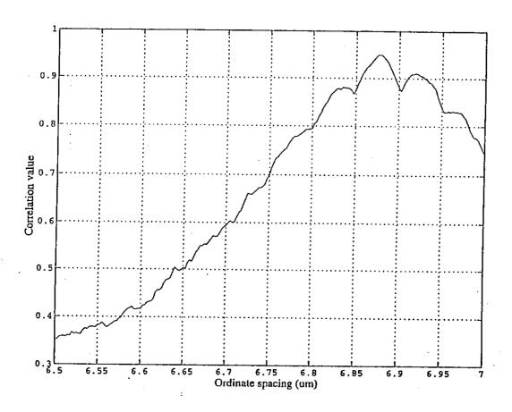
Figure 3 - Maximum cross-correlation value as a function of down sample spacing (PTB specimen).
