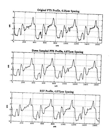
Figure 3 - Unfiltered surface profiles from the milled surface.
