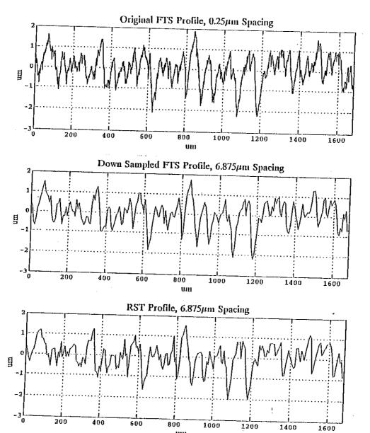
Figure 1. Unfiltered surface profiles from PTB roughness specimen
