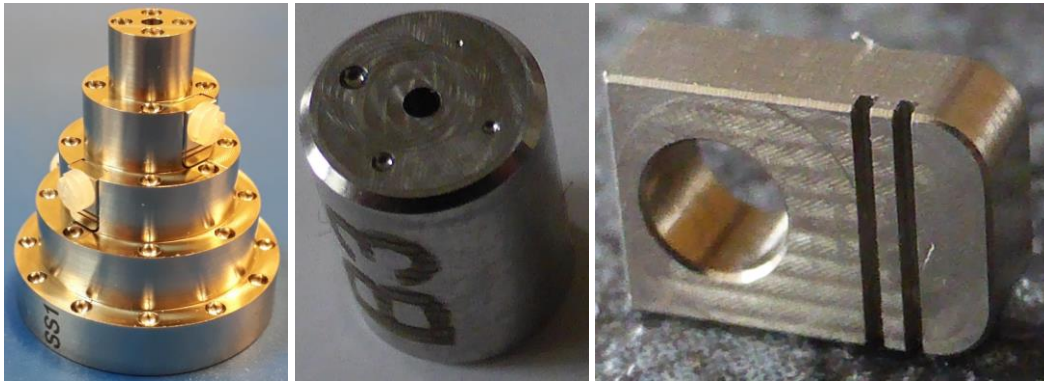
Figure 3: Stainless steel standard (left), plug with inner counterbore and sphere calottes on the top (center), insert with external grooves (right).
