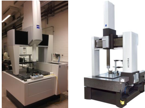
Figure 5: Zeiss Prismo CMM (left) at DTU Mekanik and Zeiss Accura II (right) CMM at LNE.
