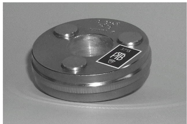
Fig.3 Photograph of a PTB multi-wave standard. The waves are found on the "belt".
