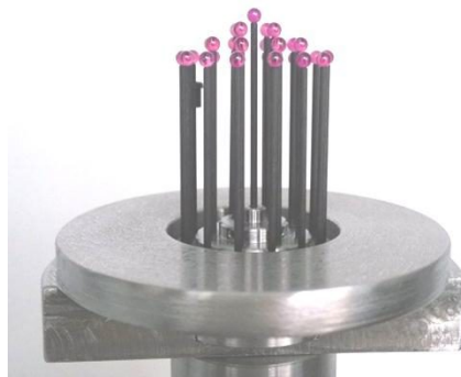
Figure 4 Tiny forest-ball. a. material object; b. CT reconstructed data (carbon fiber rods are filtered due to its low X-ray absorption coefficient)
